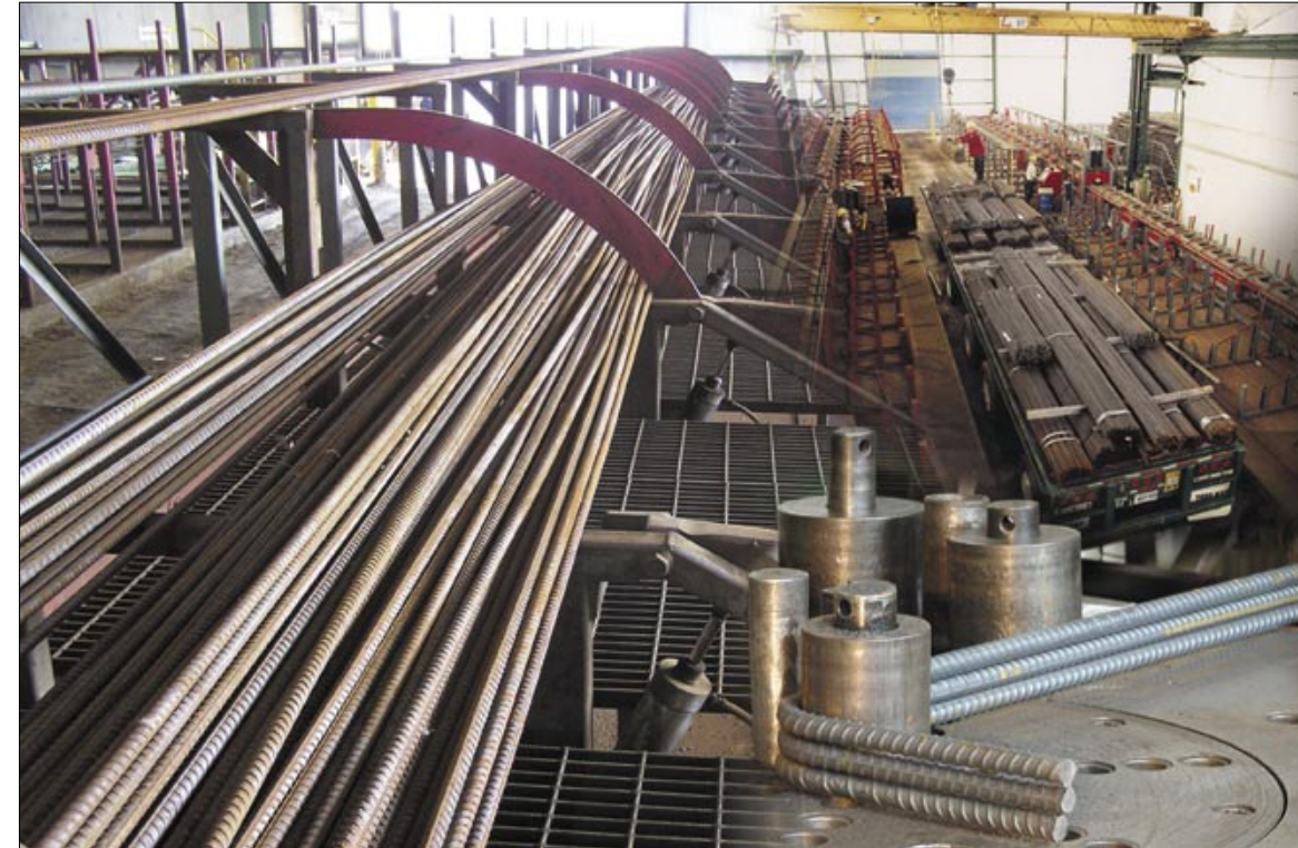
A growing operation. Salit Steel has fabricating shops in Niagara Falls (pictured above), Burlington, and Bowmanville, Ontario. The company recently added a stainless steel rebar fabricating facility in Niagara Falls, New York. By stocking several lengths of bar and using aSa's Computer Shearing and Opto-Shear Controller, Salit has virtually eliminated remnants and scrap on their larger bar sizes, according to Owner and President Steve Cohen.
